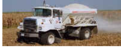
Variable Rate DGPS Equipped Lime Truck
